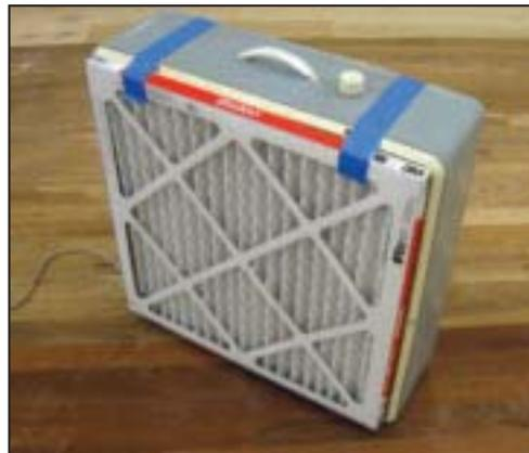
After sanding, it seems to take forever for that tiny airborne dust to settle down onto the floor; that's why many contractors wait to coat until the next day, after the dust has settled. Using a box fan with a filter taped on it—drawing in dusty air and exhausting clean air—can help speed the process, trapping airborne dust instead of just blowing it around. The number of fans and filters needed depends on the size and configuration of the area.
